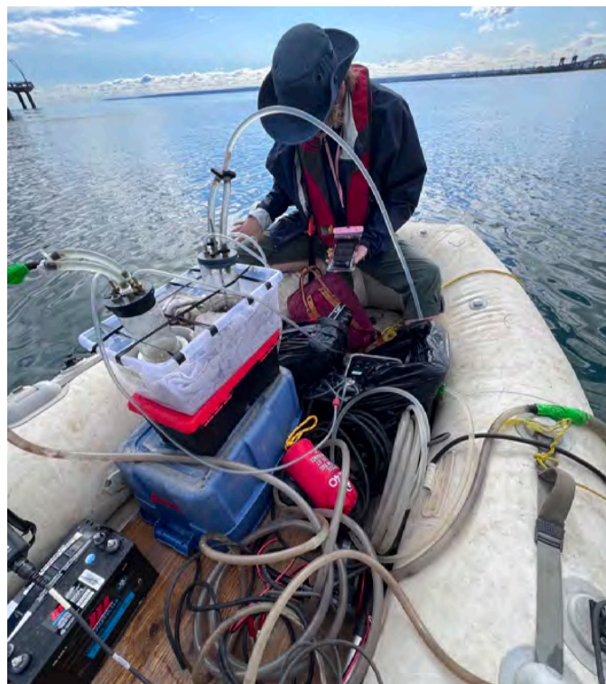
A team of ECCC scientists and Western University professors and students are using radon detectors with nearshore lake water sampling to map out areas of higher groundwater discharge along the northern shore of Lake Ontario. Credit: Kayla Bruce, ECCC.
