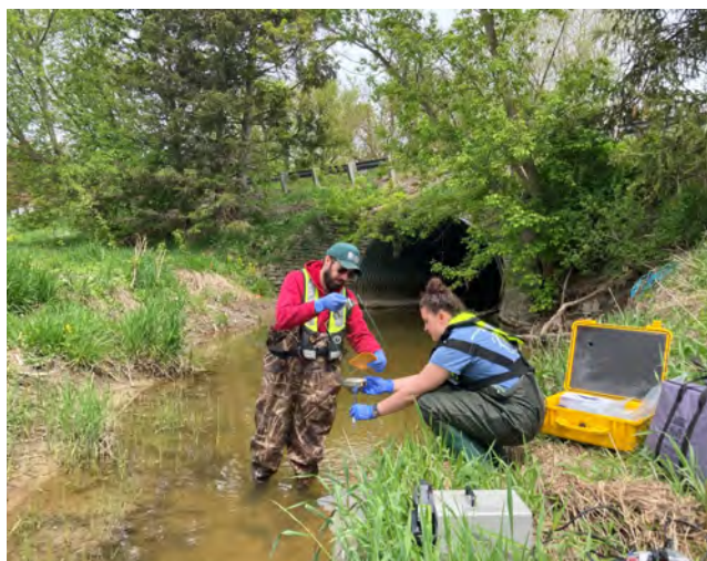
Scientists collect water from the stream surface microlayer layer for analyses of the partitioning of PFAS within stream ecosystems. Credit: Matthew Pronschinske, U.S. Geological Survey.
