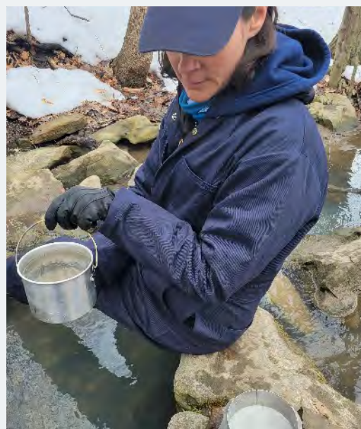
Sampling a groundwater spring for measurement of microplastic transport in groundwater in an area of urban karst (limestone/dolostone caves and cracks). Credit: James Roy, ECCC.
