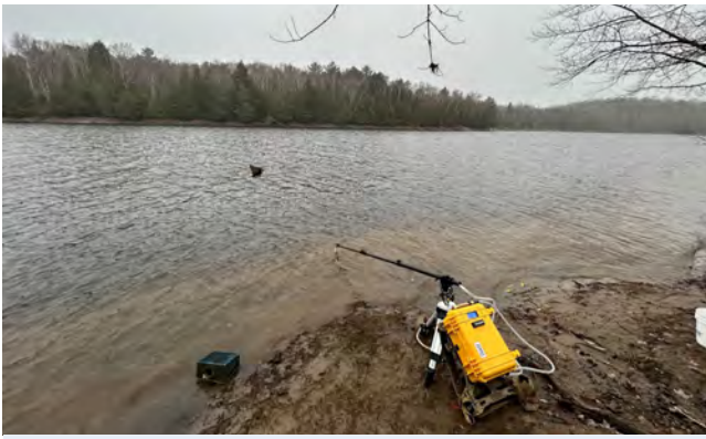
An eDNA backpack being used to collect water as part of a partnership between DFO and Mississauga First Nation to surveil for Grass Carp. Credit: DFO.
