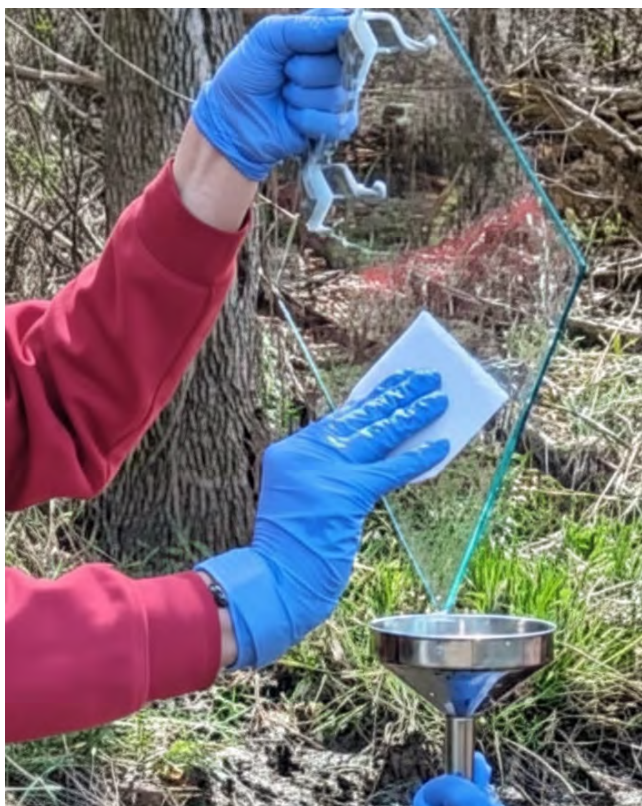
Custom method for collecting water from the stream surface microlayer layer for analyses of partitioning of PFAS within stream ecosystems. Credit: Luke Loken, U.S. Geological Survey.
