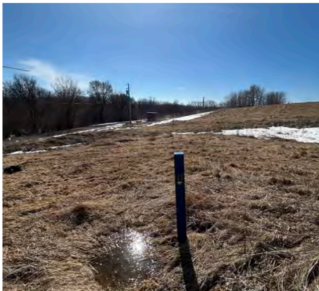
A monitoring well at the edge of a historic landfill in Ontario that was sampled for the presence of a variety of emerging contaminants, including per- and polyfluoroalkyl substances (PFAS). Credit: James Roy, ECCC.
