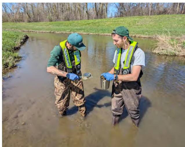
Scientists collect bed sediments using a custom hand core. Credit: Luke Loken, U.S. Geological Survey.
