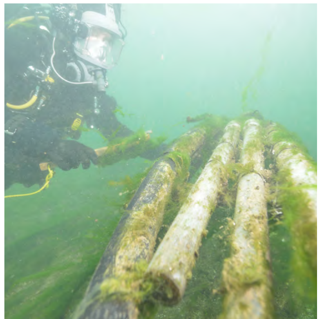
ECCC Diver performing pump wand maintenance at an ECCC Water Quality Monitoring and Surveillance in-situ sampling station in the Niagara River. Credit: ECCC/Research Support Section.
