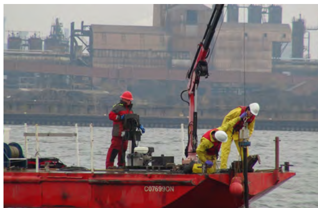
ECCC staff working onboard the CCGL GOOSE III conducting vibracore sampling near the Randle Reef Remediation Project, Hamilton Harbour Area of Concern. Credit: ECCC/Research Support Section.
