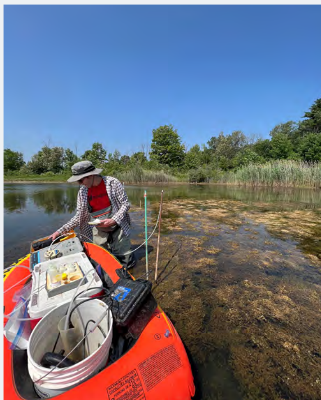
ECCC scientists sampling groundwater discharging into a shallow pond as part of an investigation into ecological exposure to groundwater impacted by mixtures of legacy and emerging contaminants. Credit: Kayla Bruce, ECCC.
