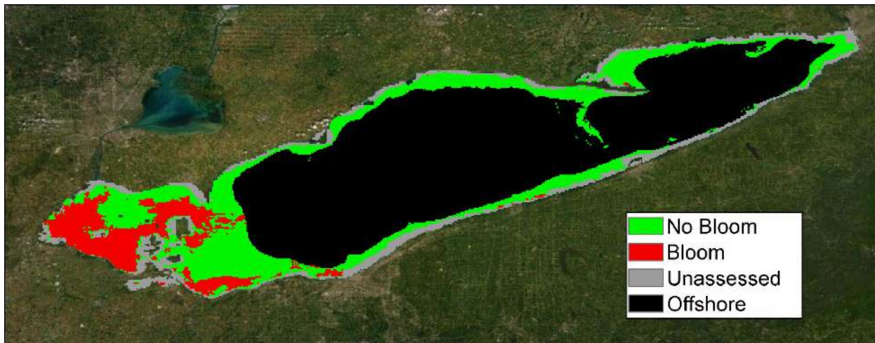
Figure 12. Lake Erie 2020 algal nearshore bloom occurrences derived from VIIRS satellite data, algal bloom occurrences (i.e., chlorophyll-a > 18 mg/m 3 and surface temperatures > 20 °C). Red areas indicate bloom occurrences (1 or more occurrences) while green areas experienced no bloom. Areas in gray were unobservable by VIIRS.
