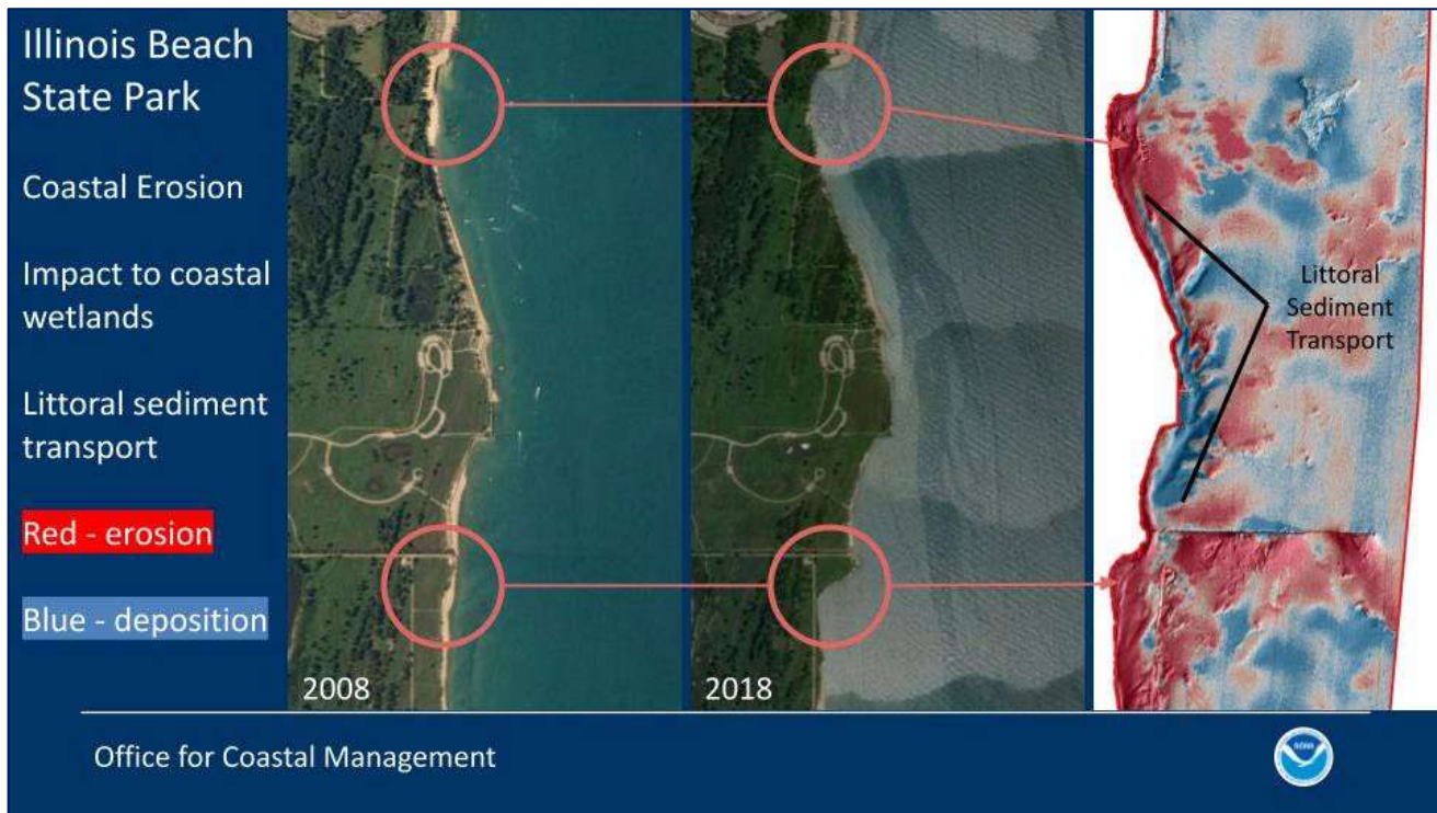
Figure 9. Images of Illinois Beach State Park. Image on left is from 2008, image in middle is from 2018, and image on right is bathymetry elevation surface difference between 2018 and 2008 with red showing areas of erosion and blue showing areas of deposition in the littoral zone. Notice the erosion nick points downstream of the hardened shorelines. Sources: Google Earth imagery and bathymetric surfaces developed from Joint Airborne Lidar Bathymetry Technical Center of Expertise (JALBTCX) topobathy lidar. Credit: NOAA Office for Coastal Management
