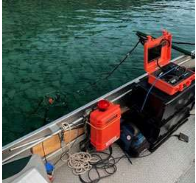
Monitoring equipment for the underwater camera used to count Round Goby and estimate the population in the lake. Source: MNRF.
