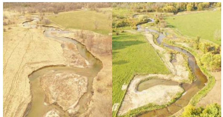
Before and after photos of bank stabilization, river restoration and channel realignment in Nottawasaga River. Source: NVCA.
