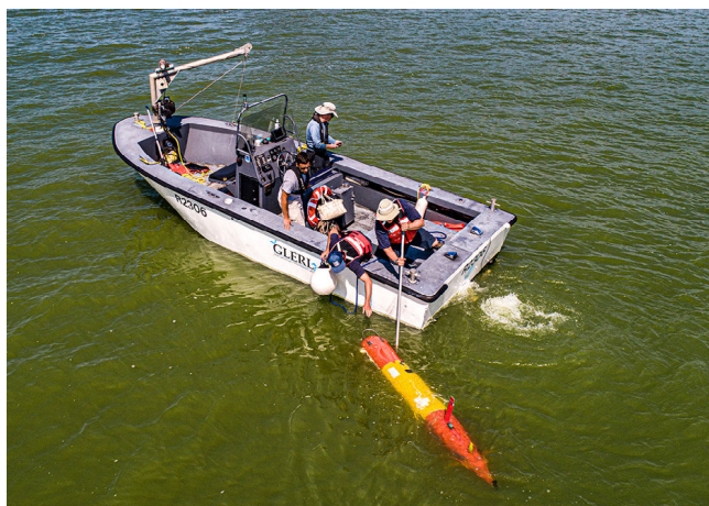
Scientists from NOAA and Monterey Bay Aquarium Research Institute aboard a NOAA research vessel deploying a long range autonomous underwater vehicle (LRAUV) in Lake Erie's harmful algal bloom. This LRAUV's mission is to map algae concentrations throughout the bloom and tell the 3rd generation environmental sample processor where to measure microcystin toxin levels. Credit: David J Ruck, Great Lakes Outreach Media
