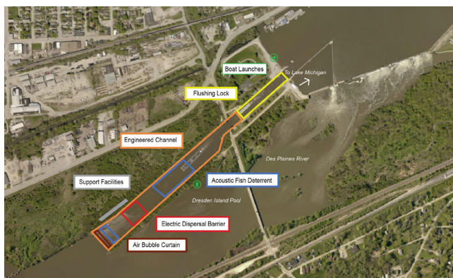
Diagram of the Brandon Road Interbasin Project Recommended Structural Plan at the Brandon Road Lock and Dam on the Illinois Waterway near Joliet, Illinois. Credit: USACE
