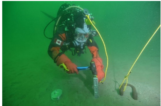
Scientist installing sampling device to extract water samples from the sand cap that isolates the contaminated sediment at the bottom of Peninsula Harbour AOC. Credit: Environment and Climate Change Canada, Water Science and Technology Directorate Dive Team
