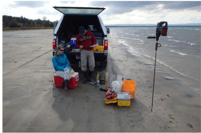
Use of a temporary drive-point system (right) to sample shallow groundwater along the shore of Georgian Bay, Lake Huron. The samples were analyzed to assess groundwater nutrient transport to the bay from septic systems. Credit: John Spoelstra, ECCC.
