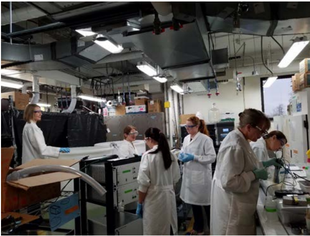
Laboratory-Based Testing Conducted by Great Waters Research Collaborative in 2018. The objective of this testing was to determine the biological efficacy of a ballast water treatment technology to the freshwater algal species Selenastrum capricornutum . Credit: Great Water Research Collaborative.
