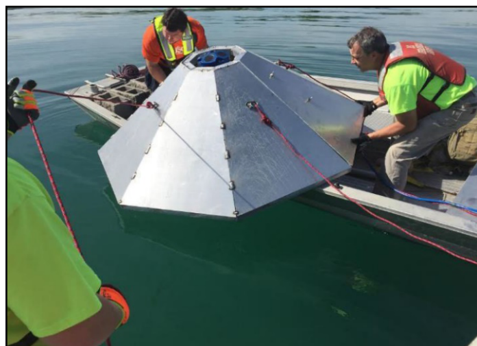
Researchers collect wave and current data at Ogden Dunes, Indiana, as part of a study to monitor movement of dredged material placed in the nearshore littoral zone. Photo: USACE.
