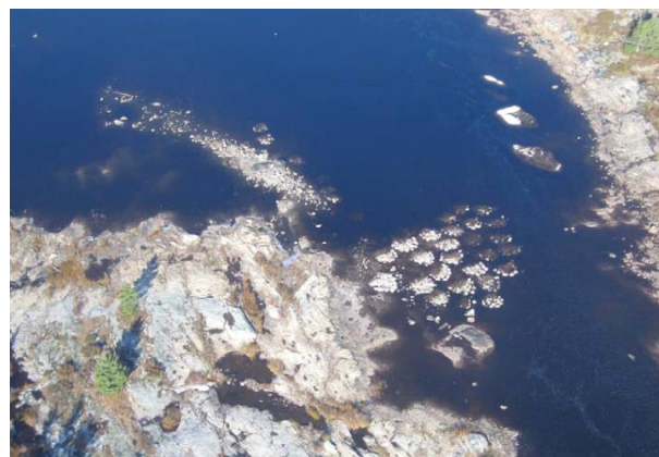
Artificial shoals and rock clusters improved Walleye spawning habitat at the Moon River basin (OMNRF).
